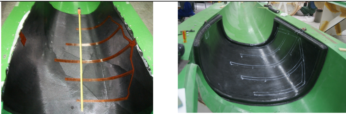
Figure 5: Design of piezo – based SHM systems.
